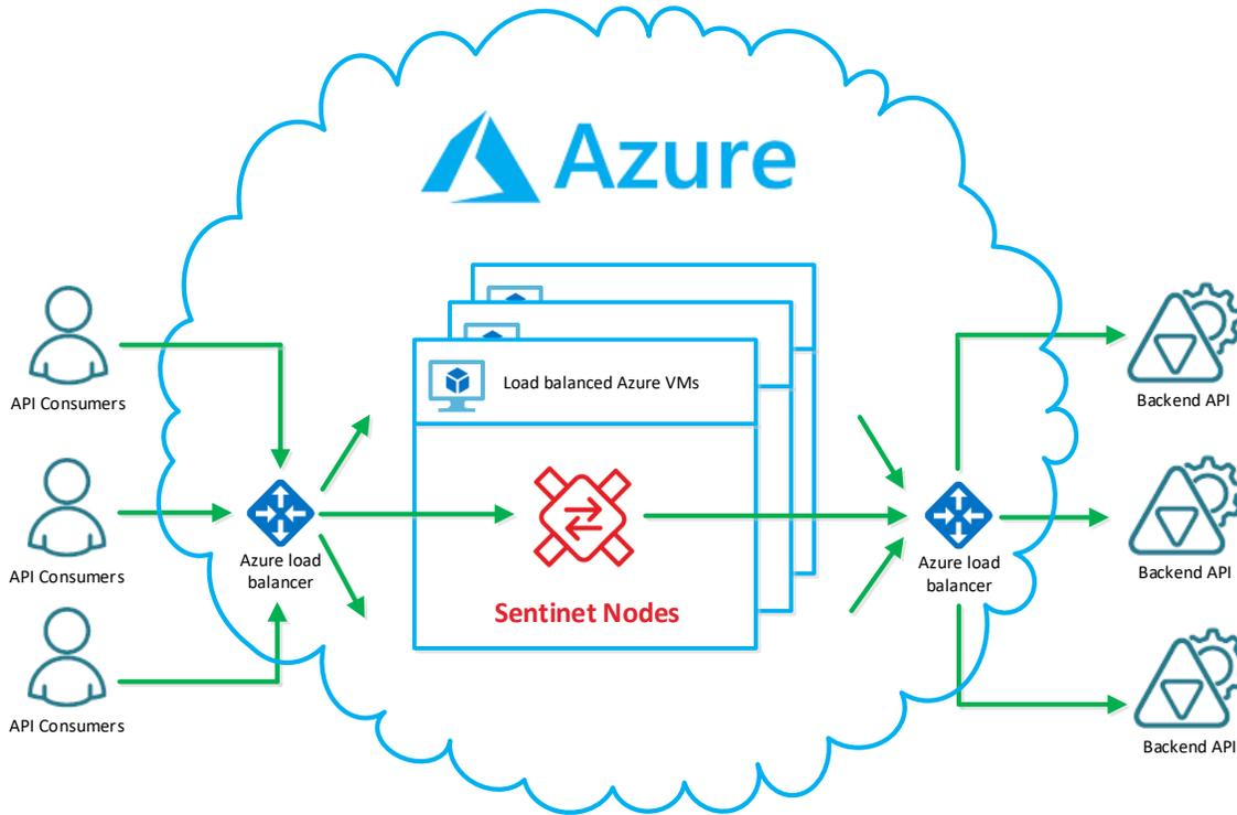
If all Sentinet components are deployed in the cloud, Sentinet is called to be in a **Cloud Model**. The diagram below shows extended version of the previous diagram.
